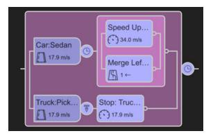
The boxes are action phases. The first action phase for each vehicle specifies the initial state of the vehicles at the start of simulation.
