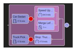
The scenario also includes an end condition. In this case, the scenario ends after a certain amount of simulation time elapses. Scenario end conditions also include a default fail condition in which the simulation ends as soon as any actor collides with another actor. If a scenario does not have an end condition, then the simulation continues indefinitely.
