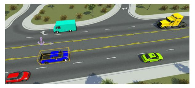
By selecting an actor and right-clicking within the scenario, you can define paths for the vehicle to follow. By default, paths snap to lanes, enabling you to quickly create complex paths such as turns and lane changes. For additional flexibility, you can change the shape of paths by modifying tangent waypoints, shift paths laterally within a lane, and specify free-form paths that go off-road or disobey traffic laws.
