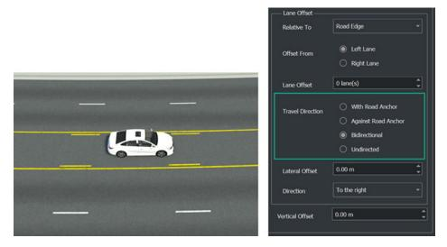
If no bidirectional lane is present in the scenario, the bidirectional lane is not close enough to the actor or is on a separate road, or the bidirectional lane is in a junction that does not have maneuvers, RoadRunner Scenario displays an error in the **Attributes** pane: This point has an unreachable forward or lane offset.
