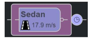
Initial action phases correspond to actors in the scenario. To add a new initial action phase, drag a new actor from the **Library Browser** into the scenario. All actors in a scenario must have a corresponding initial action phase. Deleting an initial action phase for an actor results in a simulation failure.
