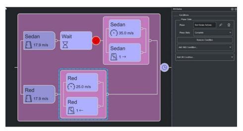
Phase state conditions enable more complex synchronization between actor actions, beyond serial and parallel execution.
