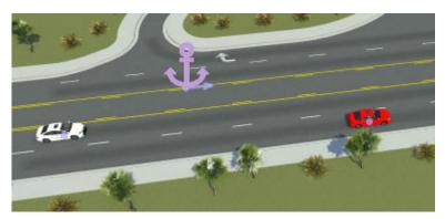
4 Set the initial speed of the lead vehicle to be slower than the ego vehicle. In the **Logic** editor, select the initial action phase for the lead vehicle. Then, in the **Attributes** pane, in the **Initialize Speed** action, set **Speed** to 10 m/s.
