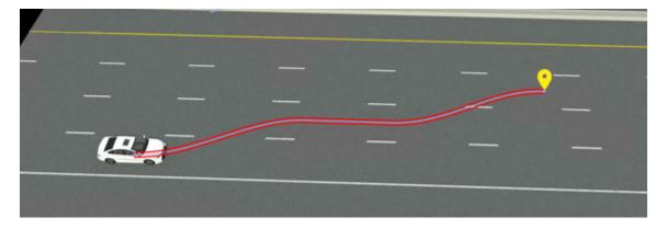
The generated path remain snapped to the lane centers. By default, lane changes take place over a maximum distance of 20 meters. To modify this distance, select the path or any segment or waypoint along it, and in the **Attributes** pane, modify the **Lane Change Distance** attribute. Lane change distances apply to the entire path. This table shows sample lane change distance values.
