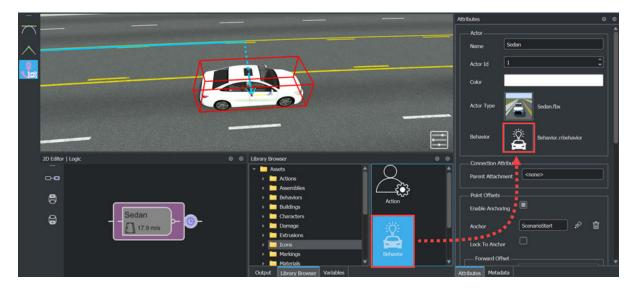
You can change or reference behavior parameters during the simulation by, in the **Logic** editor, using the Change Behavior Parameter action phase and Behavior Parameter condition respectively. For more information about behavior parameter action phases, conditions, and the **Logic** editor, see "Define Scenario Logic" on page 3-75.
