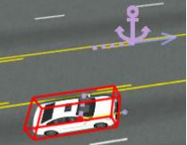
2 Add a path segment by right-clicking the adjacent lane slightly in front of the ego vehicle. RoadRunner adds a new path waypoint, selected in yellow, at the point where you clicked. The purple path segment snaps to the center of the lane and includes a lane change maneuver.
