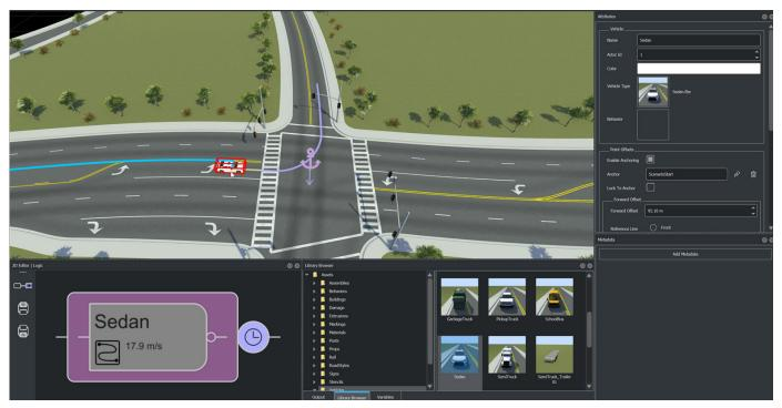
8 Place the ego vehicle for CARLA to control. Select the Compact car from the Library Browser, and drag it onto the scene. With the vehicle selected in the scene, specify a path by right-clicking to create waypoints on the roads. In this simulation, the compact car follows the same path as the sedan.
