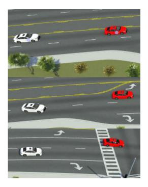
The simulation continues playing, with the ego vehicle moving forward in the lane right of the reference vehicle at the speed of 17.88 m/s.
