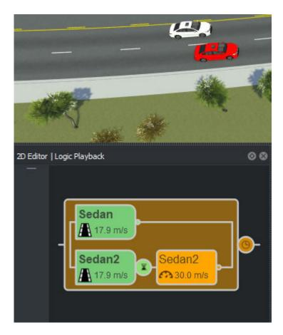
Alternatively, instead of using a Duration condition, you can use the Simulation Time condition.
