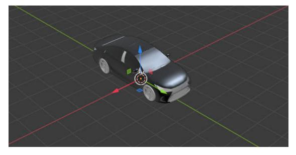
Create and assign material slots to the vehicle body. Confirm that the first material slot corresponds to the body object. For example, this image shows the hierarchy in Blender.
