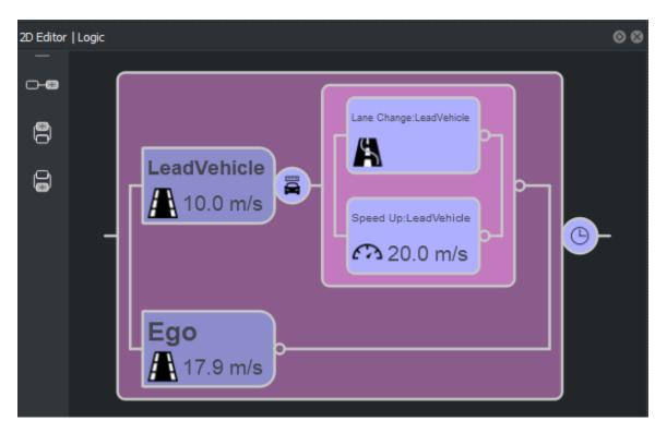
To test your scenarios, RoadRunner Scenario provides an in-editor simulation tool. From the toolbar, select the **Simulation Tool** to enable simulation controls. Using the controls in the **Simulation** pane, you can control the pacing and step size of the scenarios.
