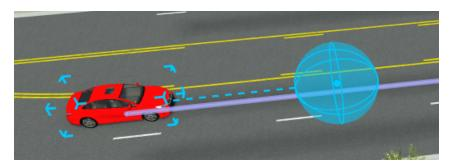
Try modifying the attributes for this condition to see how they affect the simulation. Moving the path waypoint that triggers the condition can also change the condition.
