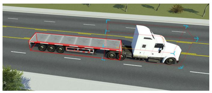
**3** You can adjust the position of the trailer, relative to attachment point on the parent vehicle, by using the Parent Attachment Point attributes of the trailer. This image shows the **Forward** offset attribute of the trailer set to 1.00 m.
