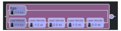
Each action occurs over the course of 2 seconds, because the added actions inherit the **Time** value of 2 from the first lateral offset action.
