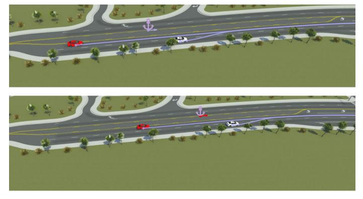
If you move a road anchor within a scenario, and then switch to scene editing mode and select the **Road Anchor Tool**, you can see the new position of the anchor reflected in the scene.
