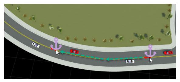
You can drag road anchors along only the road that they belong to. To move a scenario to an entirely new road, you must update the parent road anchor of each actor. For more details on changing parent anchors, see "Change Anchor Parent" on page 3-124.
