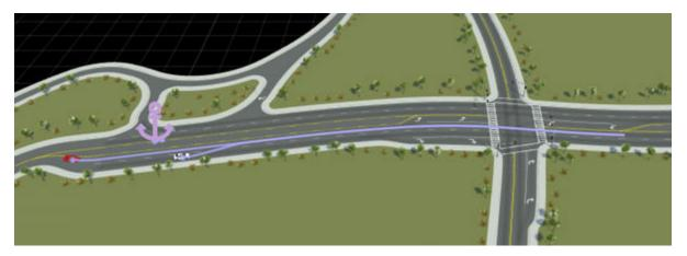
If you load the scenario into one of the default scenes that does not have a ScenarioStart anchor, such as FourWayStop, then the actors attach instead to the scenario center point, which can cause unexpected results. For example, in this figure, the actors drive off the scene and do not follow the lanes.
