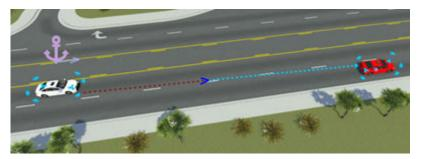
5 Simulate the scenario. The lead vehicle now does not start its lane change until the ego vehicle is closer. Depending on your initial placement of the vehicles, this scenario can end in collision.
