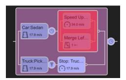
The scenario itself is also a parallel phase that consists of two serial phases: one for the truck and one for the car.
