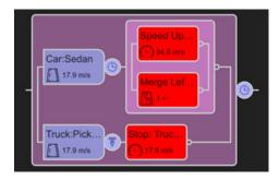
The circular nodes are conditions. These conditions trigger the next action phase to occur during simulation. For example, the car starts its next action phase after a certain amount of simulation time elapses. The truck starts its next action phase after it reaches a certain distance from a point.
