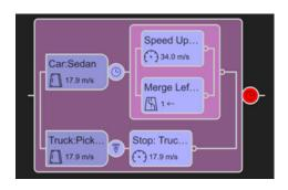
The rows containing the separate vehicle action phases and conditions are serial phases, which occur in order during simulation.
