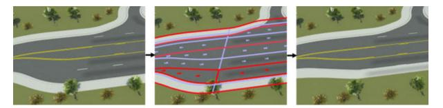
Switch back to scenario editing mode and open the TrajectoryCutIn scenario into this scene by opening the **File** menu and selecting **Open Scenario Into Current Scene**. The white vehicle no longer cuts-in, because it has no second lane to cut into.
