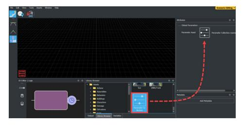
By default, RoadRunner Scenario references global parameters from the associated parameter collection asset. To initialize parameter values, in the global parameters **Attributes** pane, under **Global Parameters**, select the check boxes next to the corresponding parameter names.
