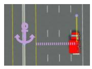
By default, each object you add to a scenario has anchoring enabled. In the **Attributes** pane for that actor, under **Point Offsets**, the **Enable Anchoring** attribute is selected. This behavior applies to vehicles and other actors, as well as to path waypoints.
