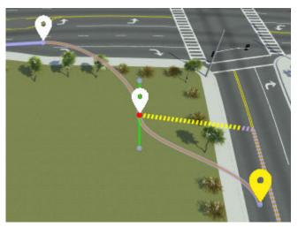
**3** Optionally refine the path further by modifying the tangent of the waypoint. For example, try rotating or extending the tangent lines.
