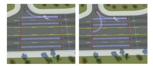
When placed in a bidirectional lane, the **Travel Direction** attribute for the actor automatically changes to **Bidirectional**. If you change the **Travel Direction** attribute of an actor to **Bidirectional** while it is in a unidirectional lane, the actor automatically relocates to the nearest bidirectional lane on the same road.
