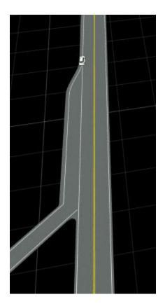
At junctions, the vehicle selects the lane that has the smallest change in curvature. For example, at this T-intersection, the vehicle goes straight instead of making a sharp turn.
