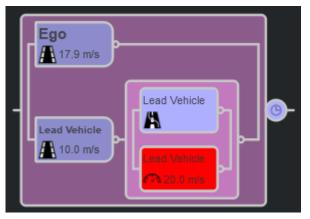
4 Simulate the scenario so far. Because the lead vehicle speeds up while performing the lane change, the scenario no longer ends in collision.
