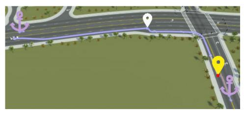
**3** Convert the added path segment to an off-road path. Select the path segment and, in the **Attributes** pane, select **Route Segment Parameters** > **Freeform**.
