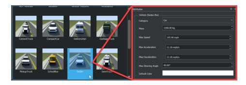
**Note** The vehicle actor attributes **Category**, **Mass**, **Max Speed**, **Max Acceleration**, **Max Deceleration**, **Max Steering Angle**, and **Default Color** do not affect the simulation, but RoadRunner Scenario stores and saves the asset values within the RoadRunner project and within exported scenarios containing vehicle actors.
