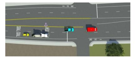
If you the change the shape of a road, the vehicles adapt to the changes while maintaining their relative positioning constraints.
