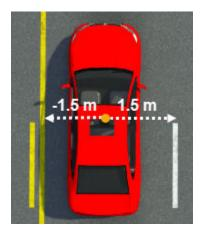
1 Right-click the Lead Vehicle initial phase and select Add Action Phase After. By default, RoadRunner Scenario sets action phases added after Initial Speed actions to Change Speed actions. Specify the action in which the lead vehicle swerves left. In the Attributes pane, set Action
