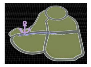
In this scenario, one vehicle cuts into the same lane as another vehicle after a specified distance. Simulate this scenario by using the SimulateScenario method. Slow down simulation pacing to 1/2 the speed to better observe the scenario.
