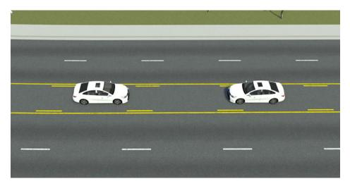
Once your scene contains bidirectional lanes, using **Scenario Editing** mode, you can place a vehicle directly in the bidirectional lane, or use a **Change Lane** action phase to simulate the vehicle changing from a unidirectional lane to a bidirectional lane. To learn more about building scenario logic and action phases, see "Define Scenario Logic" on page 3-75.
