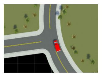
**Note** When you set the **Dynamics Type** attribute of a **Change Speed** action to With Acceleration, you must specify an appropriate sign for the value of the **Acceleration** attribute. If the sign of the **Acceleration** value does not enable the vehicle to achieve the specified target **Speed** value, the vehicle ignores the sign.
