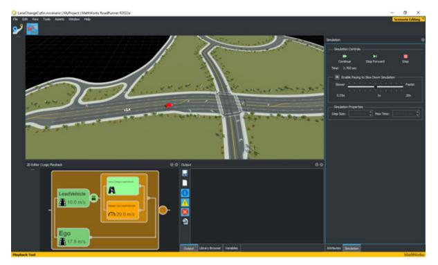
During the design and simulation process, RoadRunner Scenario provides validation feedback on your scenarios. This feedback comes in the form of visual indicators while designing and reports in the **Output** pane after simulation. Use this validation feedback to fix validation errors early, instead of waiting to catch them during the more time-consuming export process.
