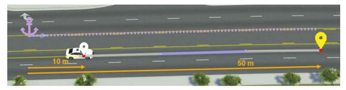
To offset the waypoint 10 meters from the vehicle, you must first change its anchor parent from the road anchor to the vehicle, and then set the offset value, by following these steps:
