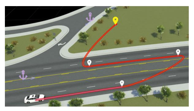
If you modify these segments to follow the road network, then they follow the road to reach the desired waypoints, leading to long and winding paths. For example, this image shows the second path segment following the road network. To reach the opposite side of the highway, the segment follows the long loop around the intersection.
