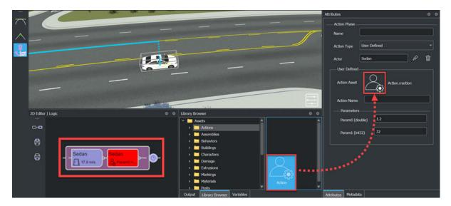
You can use user-defined action parameters to represent vehicle characteristics, such as braking force or steering angle, that you can model using actor attributes like pose and velocity. To learn more about user-defined action parameters in scenario logic, see "Define Scenario Logic" on page 3-75.
