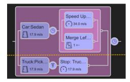
The action phases for the car in the interior box make up a parallel phase. These action phases occur in parallel during simulation.
