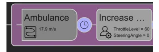
In the final action phase, the custom parameter  $\mathbf{Steering}$   $\mathbf{Angle}$  of the red ambulance is increased from 0 to 20.
