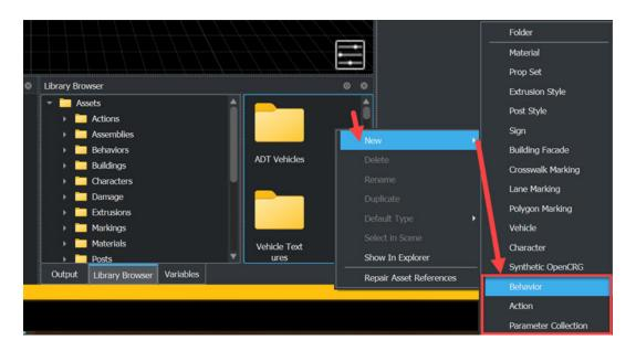
You can set initial parameter values by selecting and action, behavior, or parameter collection asset in the **Library Browser**. Then, in the **Attributes** pane, specify the parameter names in the corresponding **Name** fields, data types in the corresponding **Data Type** drop-down lists, and values in the corresponding **Value** fields.
