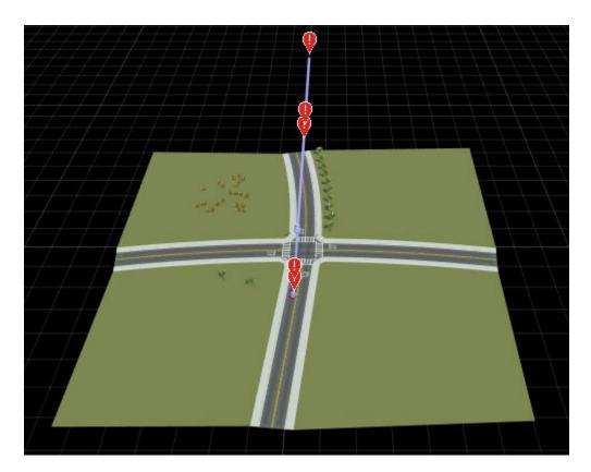
To resolve this issue, you can add a ScenarioStart anchor to the scene by using the **Road Anchor** tool.
