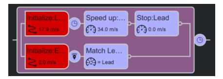
Click the two initial phases and observe the attributes of the phases in the **Attributes** pane. Both vehicles include an **Initialize Speed** action. Try changing the initial **Speed** values of the vehicles and observe the effects on simulation.
