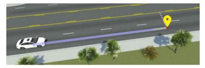
By default, paths added onto a road network snap to the center of the lane. You can then extend this path by clicking and dragging the waypoint, and the path remains snapped to the lane center.
