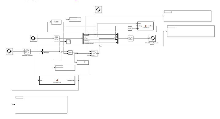
Load the Bus objects that allow the Simulink cosimulation agent to read dynamically changing vehicle information from the scenario.
