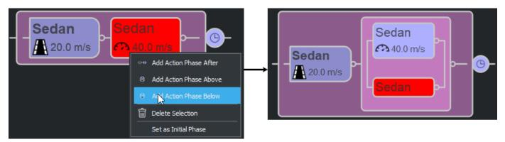
Use these parallel phases to organize your scenario logic. For example, suppose your scenario contains a chain of speed changes and lane changes. You can specify the speed change actions in one serial phase and the lane changes in another.
