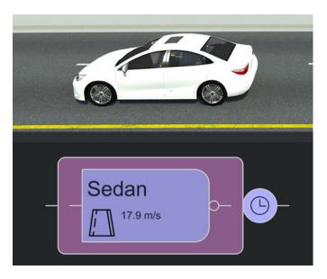
You can create more complex vehicle behavior for a scenario by adding and adjusting action phases and conditions in the **Logic** editor. To learn more about vehicle behaviors, actions, conditions, and defining scenario logic, see "Built-In Behavior for Vehicles" on page 3-145 and "Define Scenario Logic" on page 3-75.
