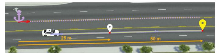
Suppose you want to set the intermediate waypoint 10 meters in front of the vehicle. Changing only the **Offset** value of this waypoint offsets it from the road anchor, not the vehicle.
